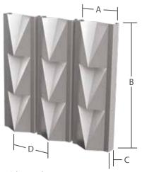
Dimensions A: Panel width: 12" B: Panel height: 12' lengths C: Panel depth: 3" inches D: Panel spacing: 13" on center Panel thickness: 0.04"
