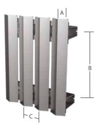
Dimensions A: Blade depth: 1.5" B: Varies based on wind loading requirements C: Blade spacing: 4" on center Blade thickness: 0.02"
