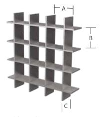
**Dimensions** A: Cell width: 2" to 12" B: Cell height: 2" to 12" D: Cell depth: 2" to 6"
