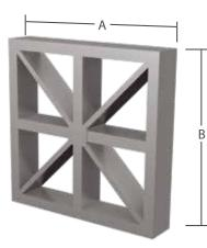
**Dimensions** A: Cell width: 1' to 7' B: Cell height: 1' to 7'
