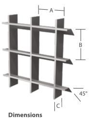
**A:** Cell width: 3" to 12" **C:** Cell height: 3" to 12" **B:** Cell depth: 3" Blade width: 0.375" 45° tilt
