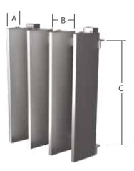
Dimensions A: Blade depth for VAC 8000: 8" Blade depth for VAC 6000: 6" B: Blade spacing: 7.875" C: Varies based on wind loading requirements
