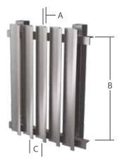
Dimensions A: Blade depth: 2.375" B: Varies based on wind loading requirements C: Blade spacing: 5" on center Blade thickness: 0.081"
