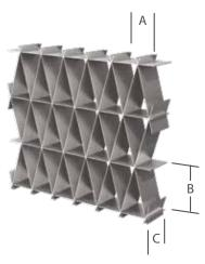
**Dimensions A:** Cell width: 7" to 16" **B:** Cell height: 2" to 6" **C:** Cell depth: 2" to 6" Bar thickness: 0.081" and 0.125"
