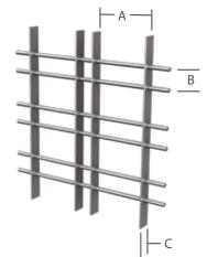
Dimensions A: Cell width: 3" to 12" B: Cell height: 3" to 6" C: Cell depth: 2"
