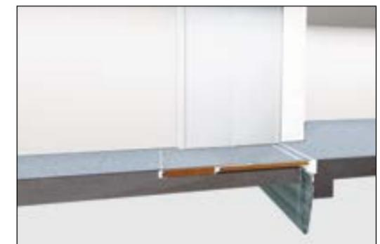
**Full Closed (During Compression)** During an event, the MACC system slides fully into the adjoining structure in the contraction (or compression) mode.
