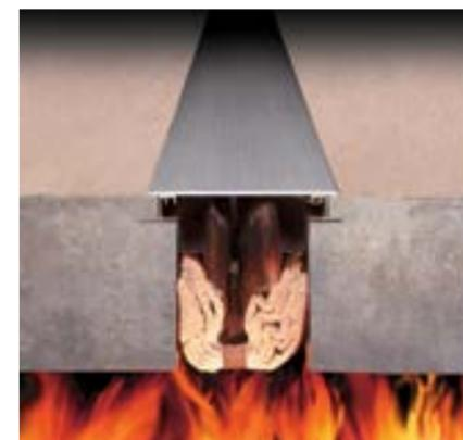
Sandwiched layers of stainless steel foil and insulation contained in a stainless steel mesh. Multiflex should be used where lateral shear is required in floor applications having a 3"-12" joint width.
